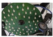
Figure 5. Hardware setup used for the acquisition. Only 9/52 LEDs are used for the acquisitions. The stereo configuration allows to get a wider view from the camera on the right whereas the camera in the center of the PCB is able to acquire near-field views of the objects.
