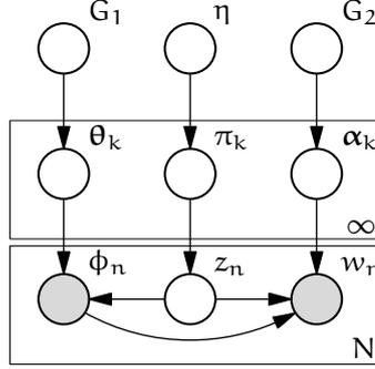
**Figure 4** The graphical model for an infinite mixture of experts.
