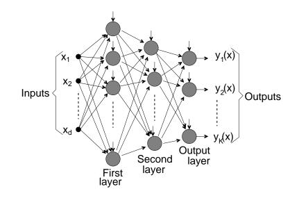
A 2-hidden layer neural network is shown above. The aim is to map an input vector  $\mathbf{x}$  into an output  $\mathbf{y}(\mathbf{x})$ . The layers may be described as:
