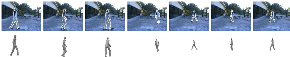
Fig. 8. Tracking a person walking in a circle. This figure shows the results of the tracking algorithm on a sequence from [15]. Overlaid is the body pose corresponding to the optimal path through the posterior distribution, the 3D model is shown below. A total of 1429 templates with 50 RVM mapping functions were used.
