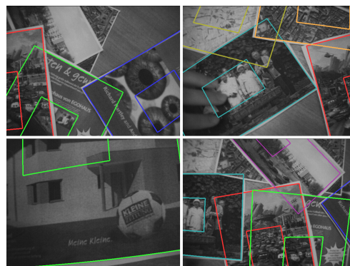
Figure 1: Four frames from a sequence demonstrating independent multiple object localisation. No frame-to-frame tracking is performed; the objects are localised in each frame. The mean total computation time per frame is 7.46ms using a single core of a 2.4GHz CPU.
