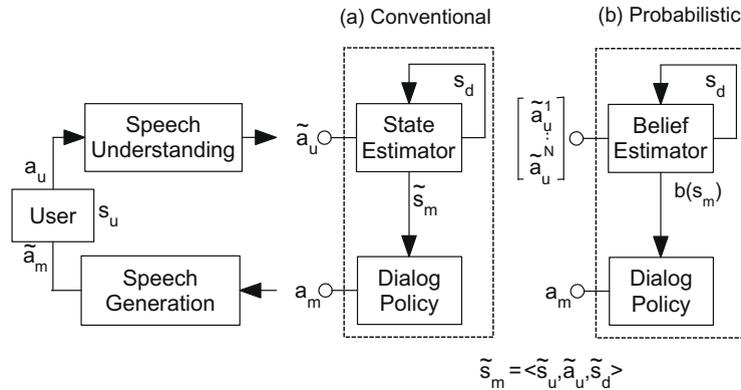
Fig. 1. Structure of a spoken dialogue system:  $a_u$  and  $a_m$  denote user and machine dialogue acts,  $s_u$  is the user goal and  $s_d$  is the dialogue history. The tilde indicates an estimate. Part (a) shows a conventional dialogue manager which maintains a single state estimate; (b) shows a dialogue manager which maintains a distribution over all states and accepts an  $N$ -best list of alternative user inputs.
