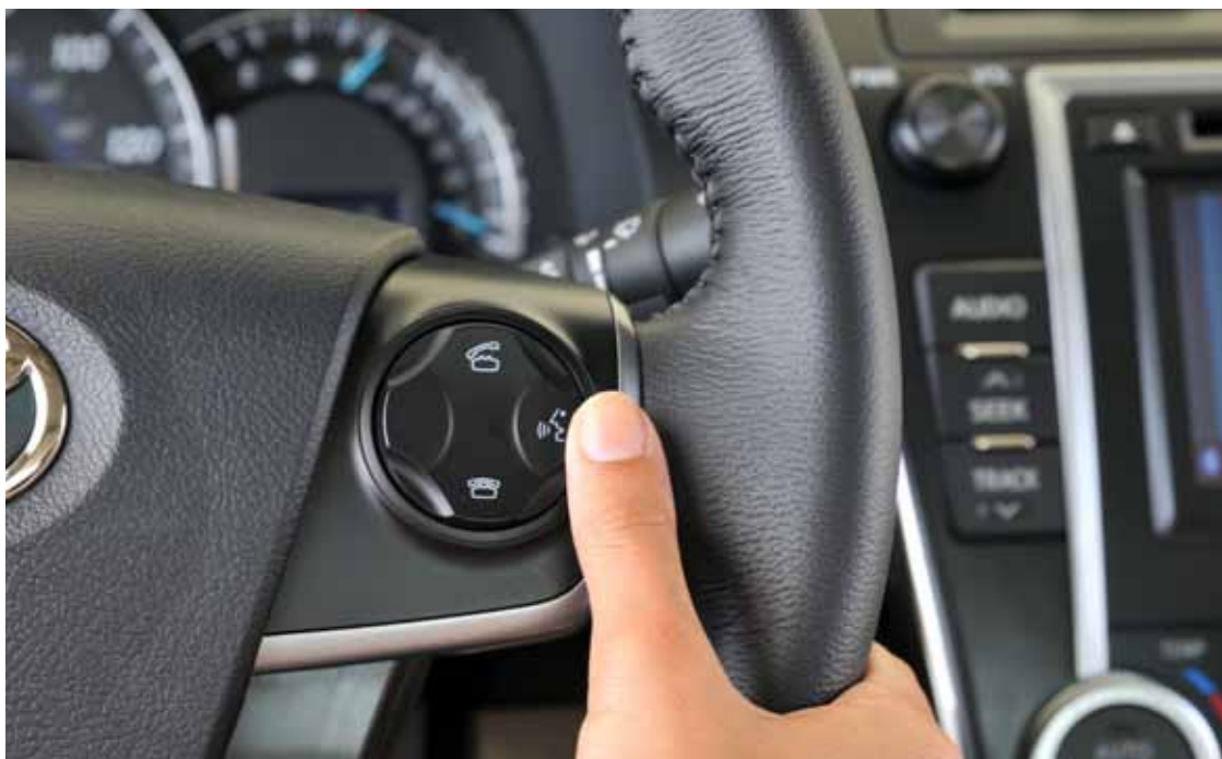
Toyota includes voice recognition technology in its most recent vehicles, accessible via the steering wheel. The system allows natural speech rather than needing to memorise and recite specific preset commands. It is linked to various multimedia functions including satnav and phone © Toyota
