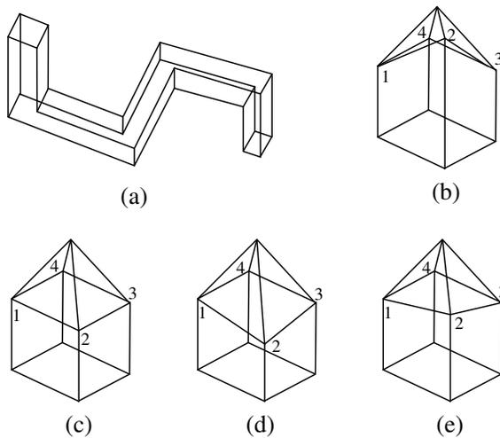
Fig. 19. (a) An object without internal faces. (b) An object with a self-intersecting internal face. (c) (d) (e) Objects with non-self-intersecting internal faces.
