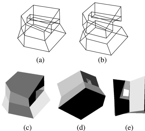
Fig. 16. (a) The line drawing of an irregular object. (b) Decomposition result. (c) (d) (e) Reconstruction result displayed in three views.
