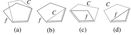
Fig. 4. Several cases where a cycle  $C$  and a real face  $f$  share two non-collinear edges and they have an overlapping region in the line drawing. (a)  $C$  and  $f$  have intersecting edges. (b)–(d)  $C$  and  $f$  have an overlapping region without intersecting edges.
