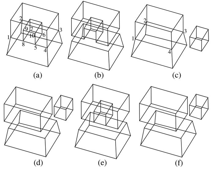
Fig. 11. (a) The original line drawing. (b) Partition result along  $C_1$  from (a). (c) Partition result along  $C_3$  from (a). (d) Further partition result along  $C_4$  from (c). (e) Partition result along  $C_2$  from (a). (f) Further partition result along  $C_3$  from (e).
