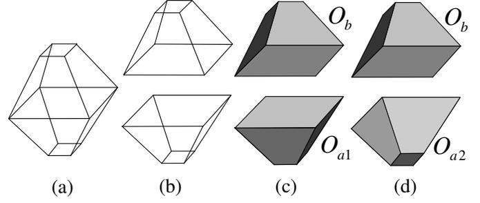
Fig. 12. (a) A line drawing. (b) Two decomposed line drawings. (c) Incompatible objects  $O_{a1}$  and  $O_b$ . (d) Compatible object  $O_{a2}$  and  $O_b$ .
