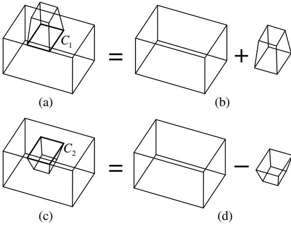
Fig. 7. Union and subtraction that generate internal faces. (a) A manifold. (b) Two manifolds whose union results in the manifold in (a). (c) Another manifold. (d) Two manifolds, with which the subtraction of the smaller one from the bigger one results in the manifold in (c).  $C_1$  and  $C_2$  are two internal faces.
