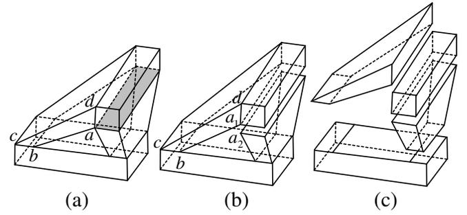
Fig. 8. An example of decomposing a line drawing along its internal faces. (a) The line drawing with one internal face shaded. (b) The correct partition along this internal face. (c) Partitions along the four internal faces. The hidden edges are shown in dashed for easier observation.
