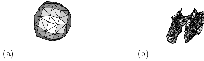
Figure 5.3: (a) Octree sampled sphere; (b) manually sampled thyroid from 3D ultrasound frames. Both meshed using Delaunay triangulation with compatibility checks.
