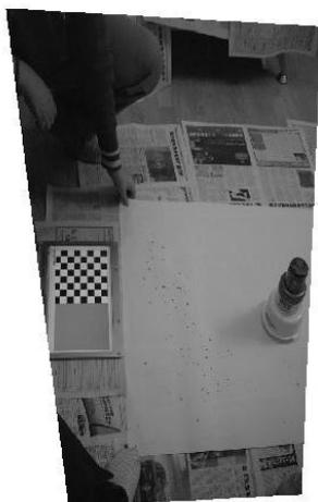
Figure 10: View of Figure 9’s scene rectification as if photographed from overhead.
