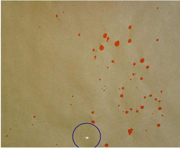
Figure 15: Rectified image of experimental multi-spot blood spatter. Note that the spatter emanated from a circular source located in the middle of the image, at the bottom edge.
