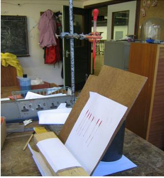
Figure 5: Apparatus used to collect experimental data of red liquid impacting a surface at a range of angles.
